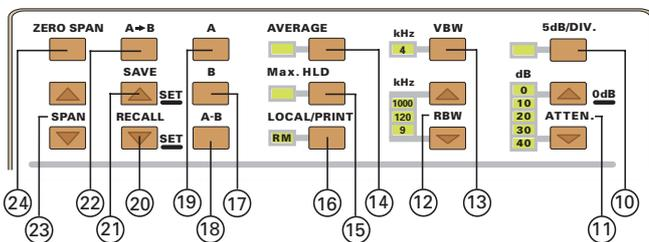
**(13) VBW** – Pushbutton with associated „4 kHz“ LED
